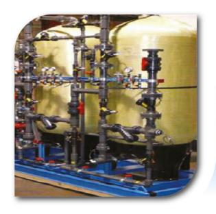
There are three ways in which ion-exchange technology can be used in water treatment and purification: first, cation-exchange resins alone can be employed to soften water by base exchange; secondly, anion-exchange
